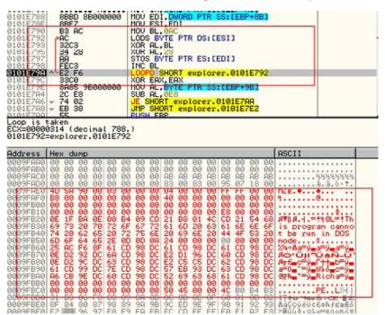
Figure 2. Decryption of the embedded binary in TROJ\_PPDROP.EVL
