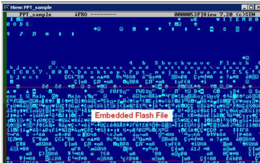
Figure 1. Embedded Flash file in TROJ\_PPDR0P.EVL
