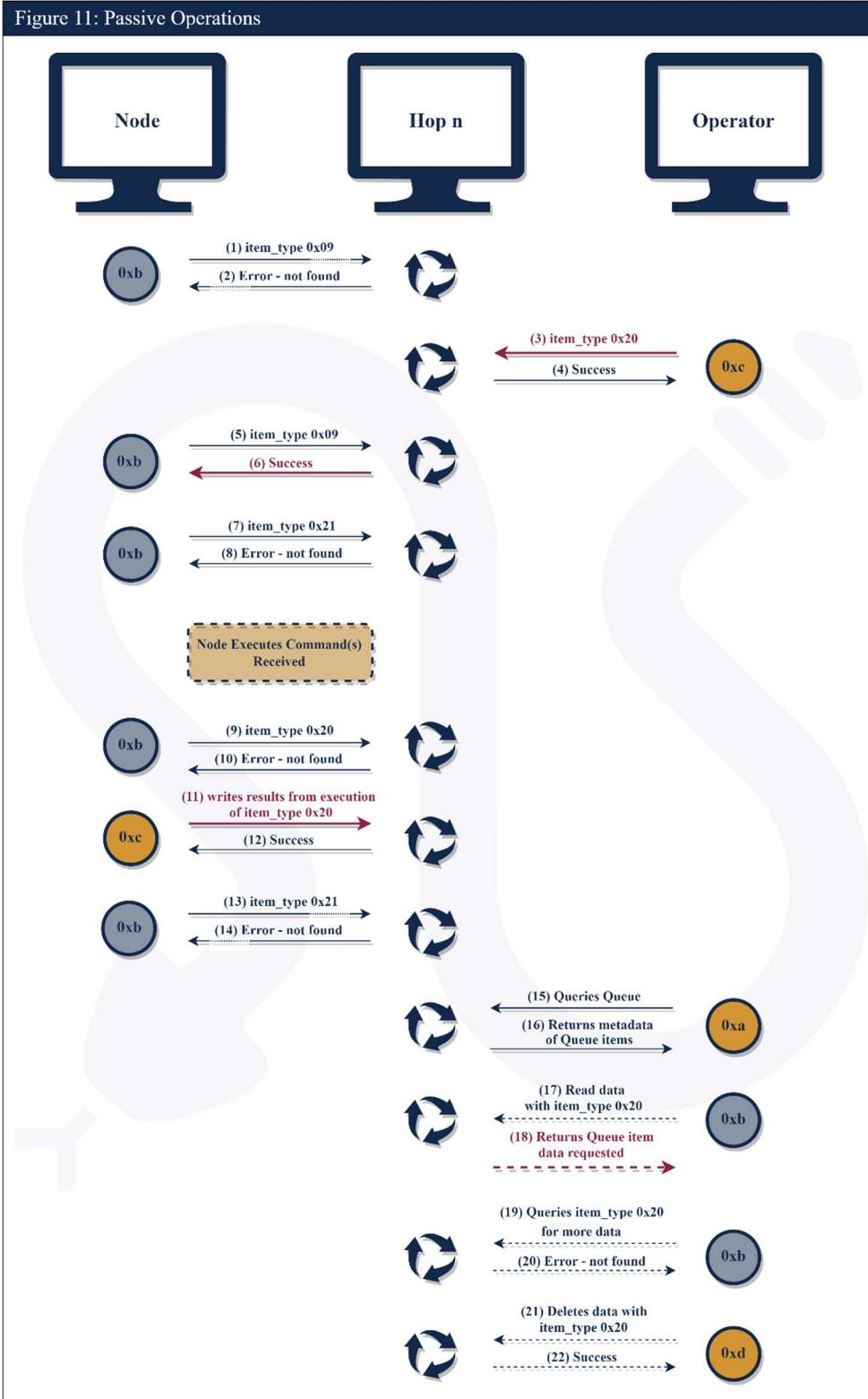
To illustrate how Passive operations are conducted between the end points, the operator, and the hop points in between, see the diagram above, which is explained further by the following steps:<sup>39</sup>
